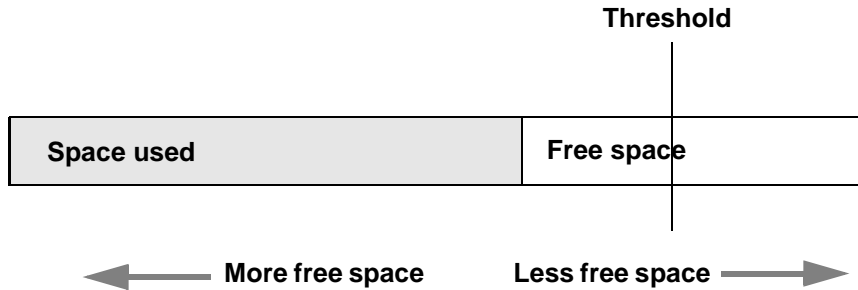
Figure 17-1: Log segment with a last-chance threshold
