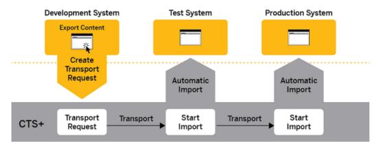
After exporting a package or application from the development system, the administrator creates a transport request in CTS and attaches the export archive. The administrator releases the transport request , and starts the import for the test system. After the import into the test system, CTS forwards the transport request to the queue of the next connected system, the production system. After a successful test, the administrator starts the import for the production system.
