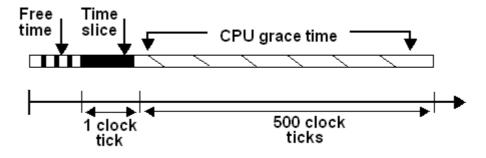
At periodic yield points, the task checks to see if the time slice has been exceeded. If it has not, the task continues executing. If it has, the task voluntarily yields the engine within the cpu grace time; if the task had not yet fulfilled the client request, the task goes to the end of the run queue. If there are no other tasks in the run queue, the server grants the task another processing interval.
