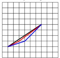
The ST\_Equals method considers the black and red lines to be equivalent within tolerance, and the red and blue lines to be equivalent within tolerance but black line and the blue line are not equivalent within tolerance. ST\_Equals is not transitive.
