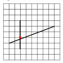
Setting the tolerance to grid size (the default), however, causes the intersection point to be inside the thick diagonal line. So a test of whether the intersection point intersects the diagonal line within tolerance would pass:
