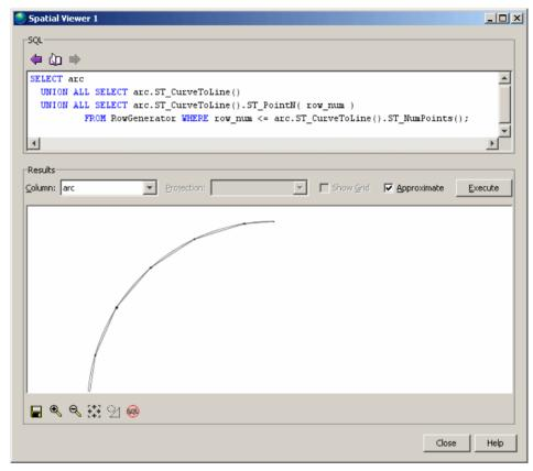
Notice how the arc is broken into a sequence of linestring. Since relative tolerance was set to 1%, each line segment shows up as a line that bows in from the true arc. The maximum distance between the interpolated line string and the true arc is 1% of the radius of the arc.
