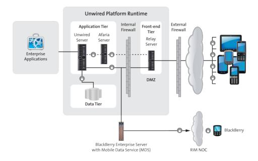
The Sybase Unwired Platform runtime landscape provides common architecture used to deploy OData SDK applications using the Online Data Proxy option.
