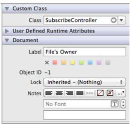
This tells Interface Builder the class of the object to allow you to make connections to and from the File's Owner.
