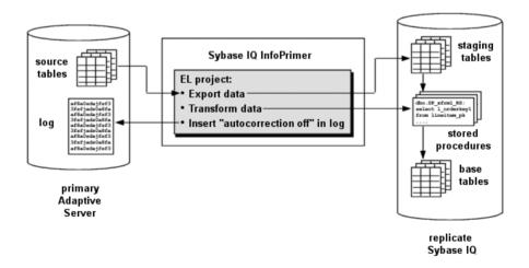
**4.** The Replication Server replicate database connection is resumed, and Replication Server processes any further changes to marked primary database tables using the staging tables and transformation stored procedures on the replicate SAP IQ database.
