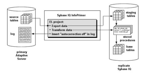
**4.** The Replication Server replicate database connection is resumed, and Replication Server processes any further changes to marked primary database tables using the staging tables and transformation stored procedures on the replicate Sybase IQ database.
