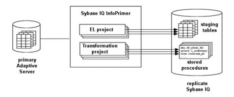
**2.** In your Replication Server instance, use the **stage\_operations** connection parameter to configure the replicate database connection to stage operations for the tables specified in your EL project.
