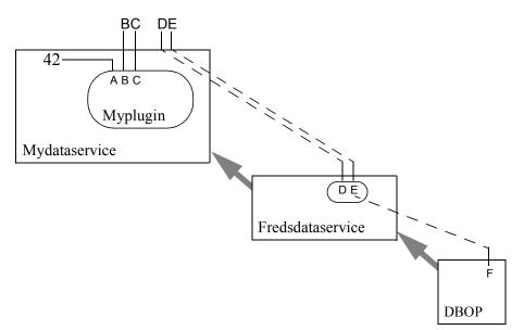
To set up Myplugin and Mydataservice, you only need to know about the parameters required by Fredsdataservice; Fredsdataservice is responsible for collecting any parameters required by its input sources (in this case, DBOP).
