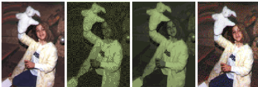
Original Image Image on a 4-gray device (Palm III) Image on a 16-gray device (Palm V) Image on a 216-color device (Pocket PC, Palm IIIc)
